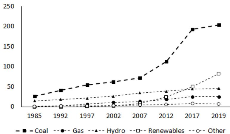
Figure 1: Capacity Expansion in Power Generation ('000 MW), by Fuel Type (Source: CEA Executive Summary on Power Sector Oct 2019)
